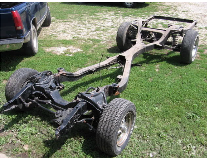
Nader didn't focus solely on Corvairs and VWs. This GM X-frame was said to split in half on impact.
