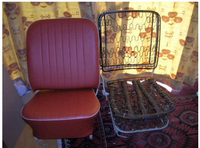
Volkswagen Beetle seat frames were susceptible to breakage causing driver and passenger ejection.
