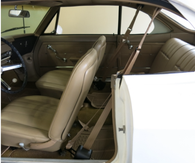
Left: Morris Classic Concepts prototype 3-point retractable seat belts as installed by John Porterfield.
