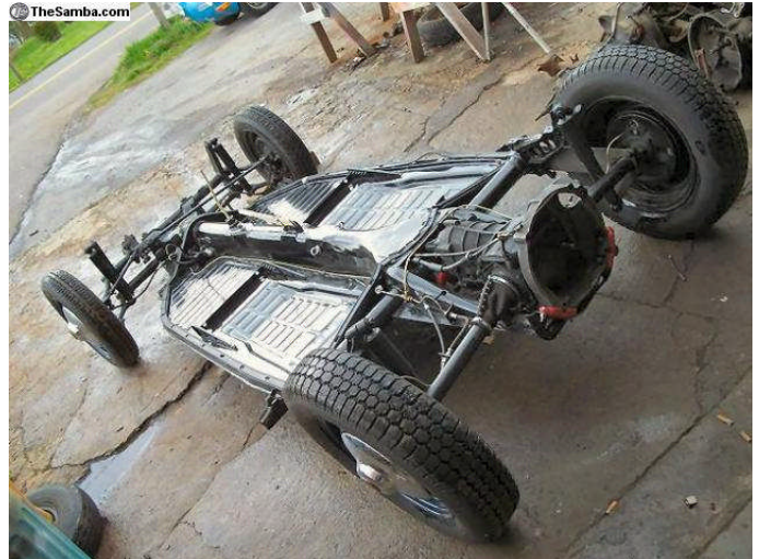
The swing axle suspension on early VW Beetle was blamed for instability and rollovers.
