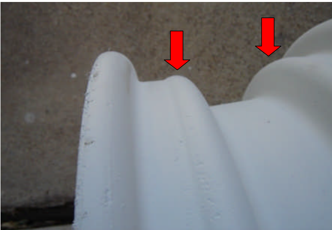
Prior to Oct. 1967, VW wheels did not have these safety beads to prevent air out with tubeless tires.
