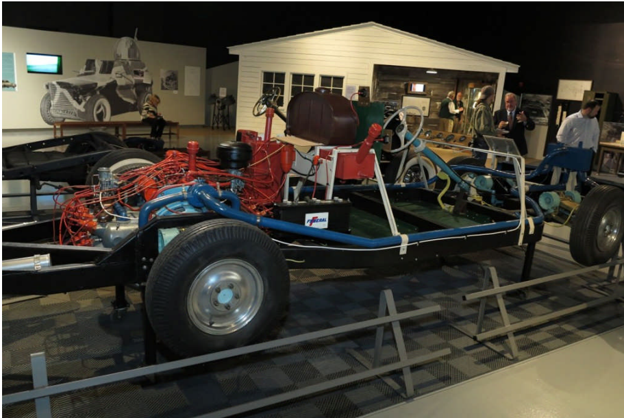
At the AACA Museum. Prototype Tucker chassis. This mule was built while Tucker was still experimenting. Note the transverse H-6 engine in the rear, which is different than the set-up used in the final version.
