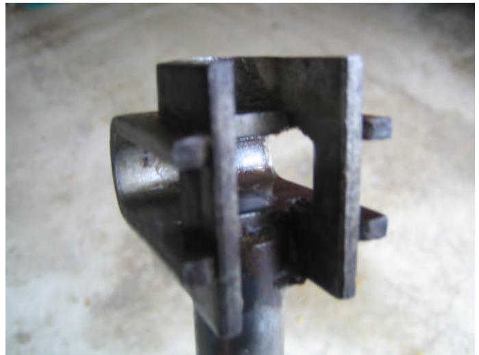
1966-1969 shift rods have a fabricated steel end which can be re-used. Note the empty "socket" at the top of the piece.
