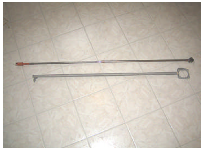
The new stainless steel shift rod laying beside the reconditioned shift tube.
