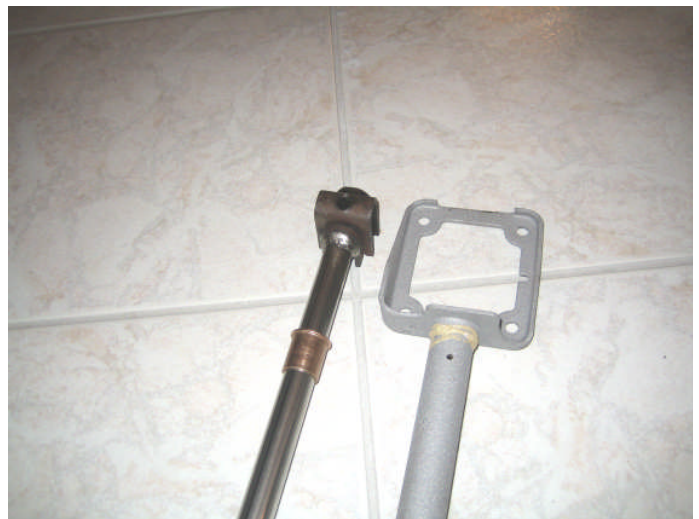
Left: Stainless steel tube welded to the fabricated end. Right: Factory shift tube, sandblasted and painted.
