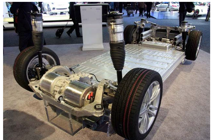
Electric motor is in the rear. Modular battery pack is contained in the floor of the passenger compartment.
