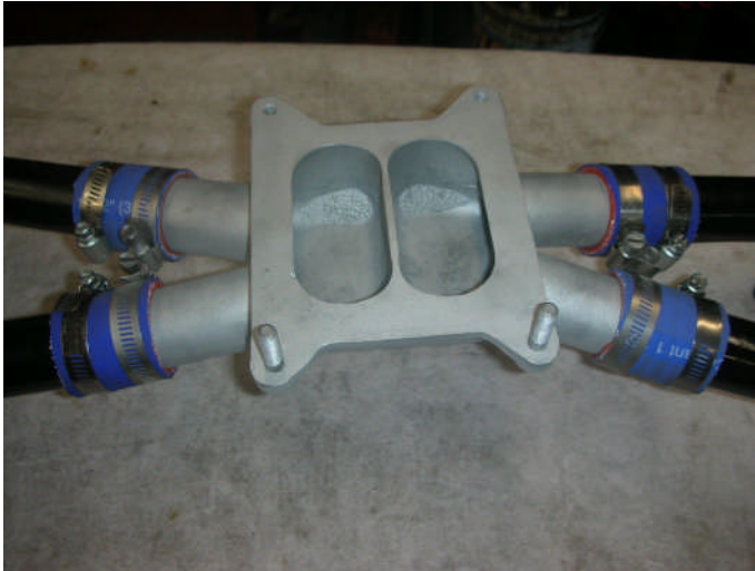
Top side of the IECO center-mount four-barrel manifold. Note the divider in the middle of the plenum.
