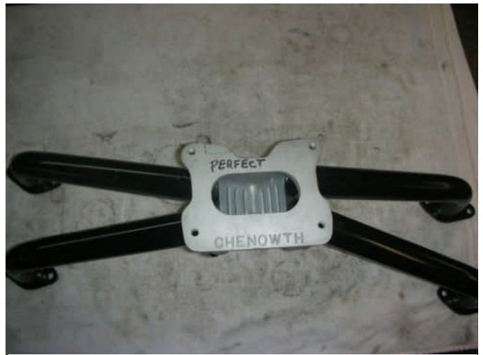
Above: A 4-barrel intake manifold manufactured by Chenoweth. Note the lack of the center divider in the 4-barrel manifold's plenum.
