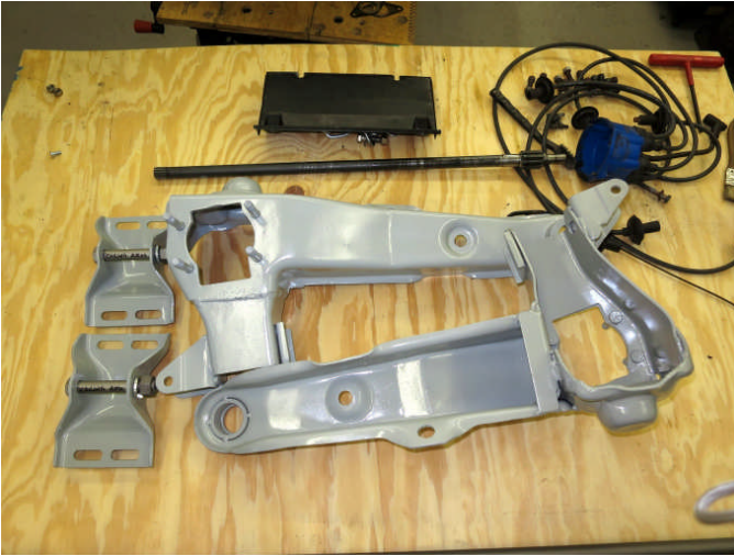
All suspension components were bead blasted and repainted. Trailing arms were reinforced and gusseted.
