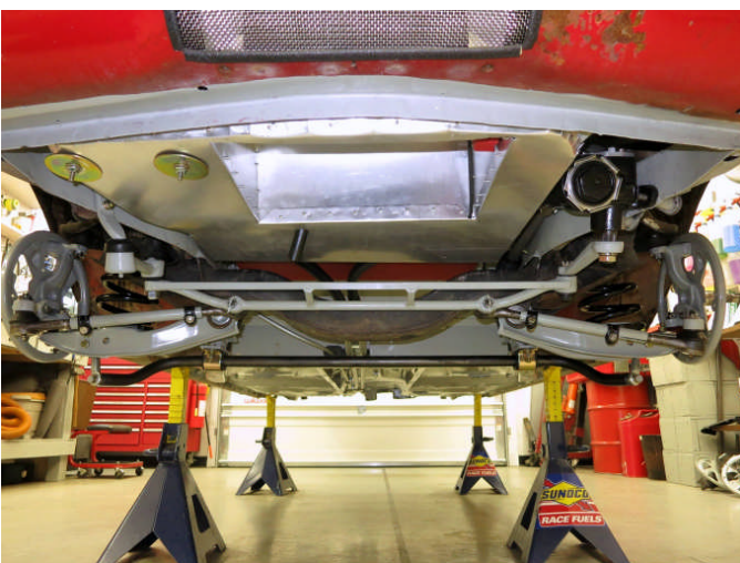
Front suspension. Drag link is trussed for rigidity. Oil cooler case made from sheet aluminum.
