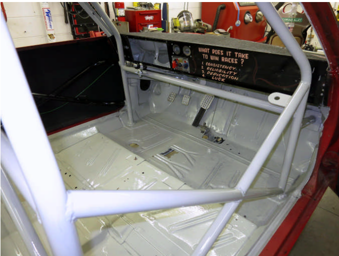
Interior painted with Rustoleum Industrial paint. Silver gray makes it easy to see any debris on floor.
