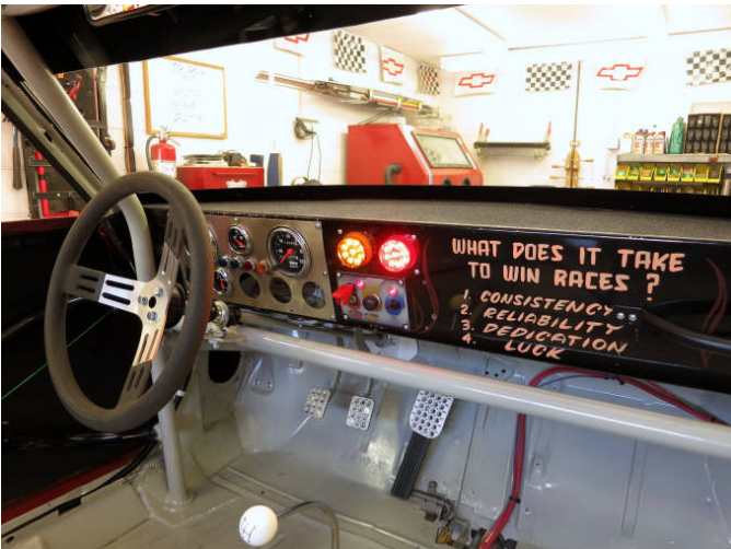
Instrument panel rebuilt with high quality gauges and switches. Entire electrical system rewired.
