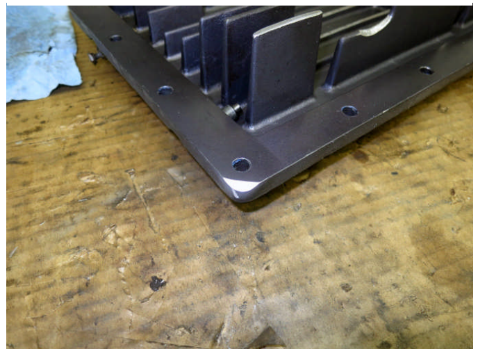
Edge of aluminum oil pan beveled slightly to enable pan to be separated from crank case more easily.
