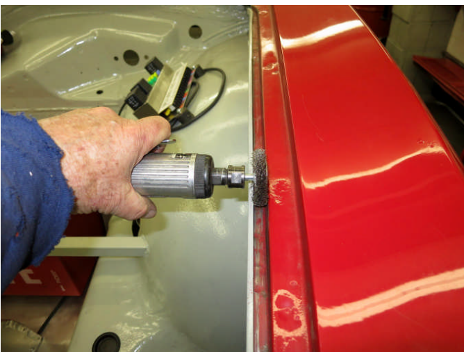
Rick removed weather stripping with a home-made scraper and then used a wire wheel on a die grinder.
