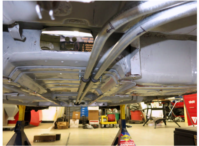
Underside. After. The tubes are oil cooler lines which Rick fabricated from electrical tubing.
