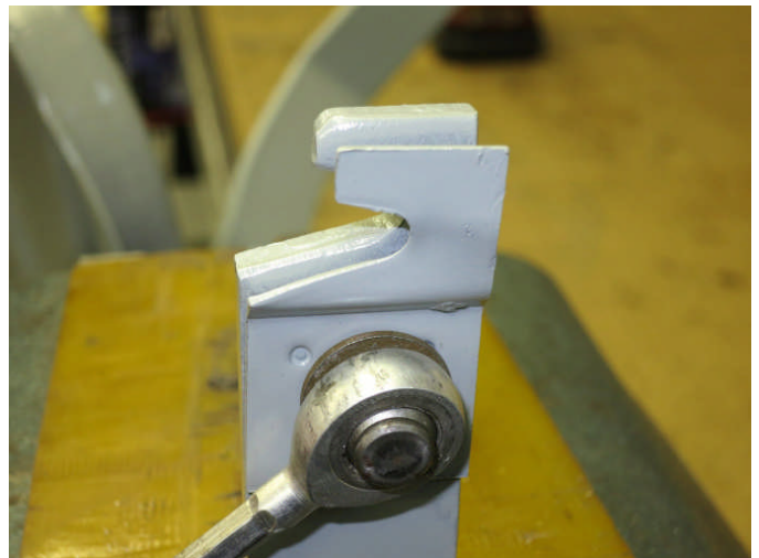
1965 clutch pedal lever modified to accept heim-jointed 1969 clutch cable. Does not affect pedal effort.
