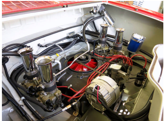
Engine: After. AN fittings on all fuel and oil lines.
