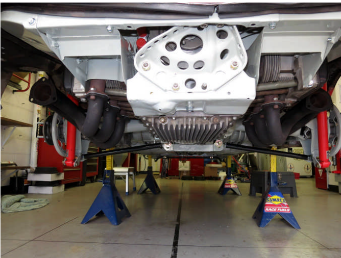
Engine mount drilled out to save weight.
