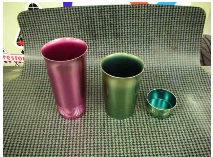
Rick fabricated his carburetor velocity stacks from these old-fashioned aluminum beverage cups.
