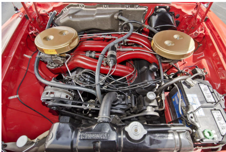
1961 Chrysler 300G cross-ram intake manifold with two four barrel carbs.
