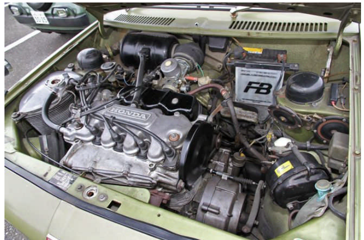
The finned container on the left is the oil sump.
