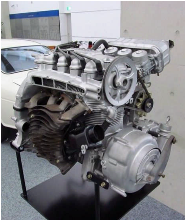
4-carb "99" version of the Honda HT 1300 engine
