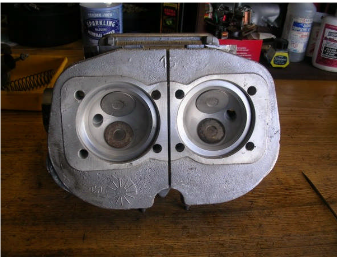
Cylinder head with hemispherical combustion chambers
