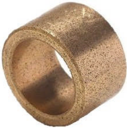
True Oilite bushings have a flecked appearance like this one. If shiny, it may have been machined improperly.
