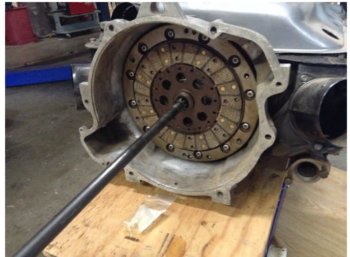
Here's the transmission input shaft inserted into the bushing.
