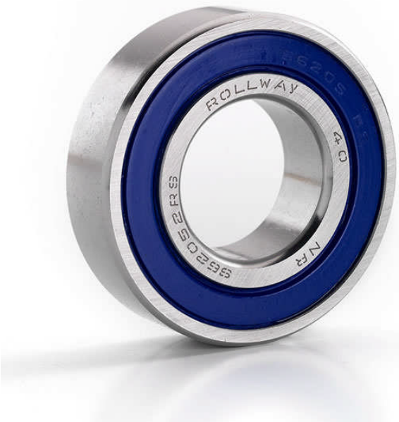
A heavy duty sealed ball or roller bearing would seem to be the best solution. They work well in applications where the pilot bearing is installed in the center of the flywheel instead of the crankshaft, but they are too big to fit in a Corvair crankshaft!
