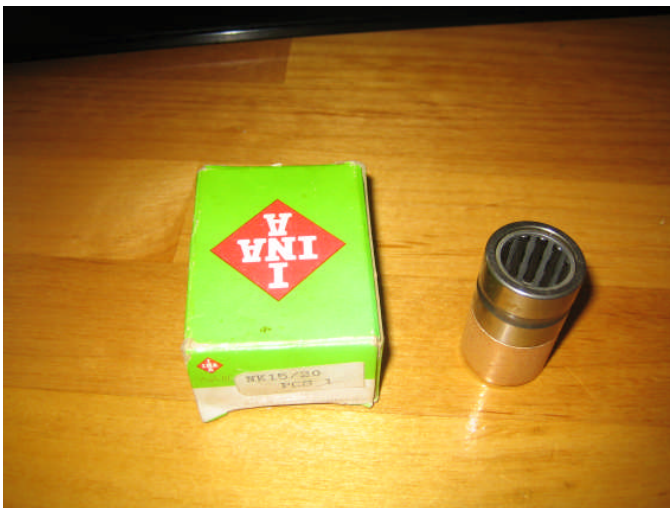
INA brand NK15/20 needle bearing, stacked on top of a Clark's Oilite pilot bushing, is just a silly millimeter longer.
