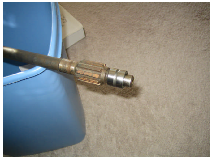
Here is the NK15/20 bearing on a Corvairster transmission input shaft. Risk: Bearing failure can take out the input shaft.
