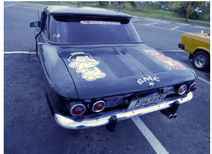
Vents once helped cool a horizontally opposed six-cylinder gas engine.
