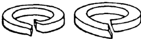
Figure 14 Helical spring washers (aka "lock washers")
