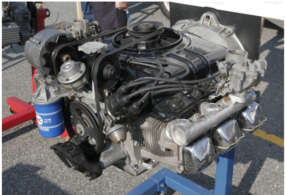
The assembled engine on a test stand. Note the individual valve cover for each cylinder. This is not the experimental overhead cam engine!
