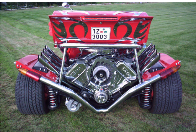
Wild trike with Tatra air-cooled V8! Centrifugal blower.
