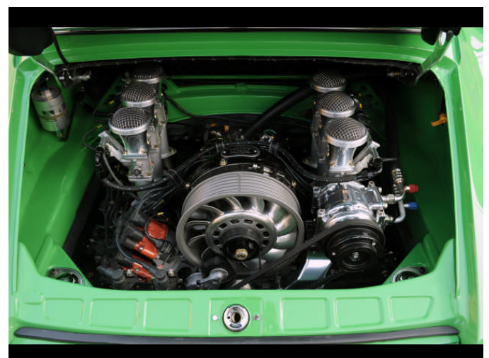
Air-cooled Porsche 911 engine uses axial blower.
