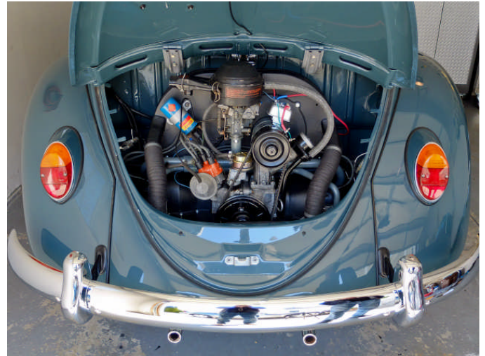
You can't see this VW's blower. Inlet faces the front!
