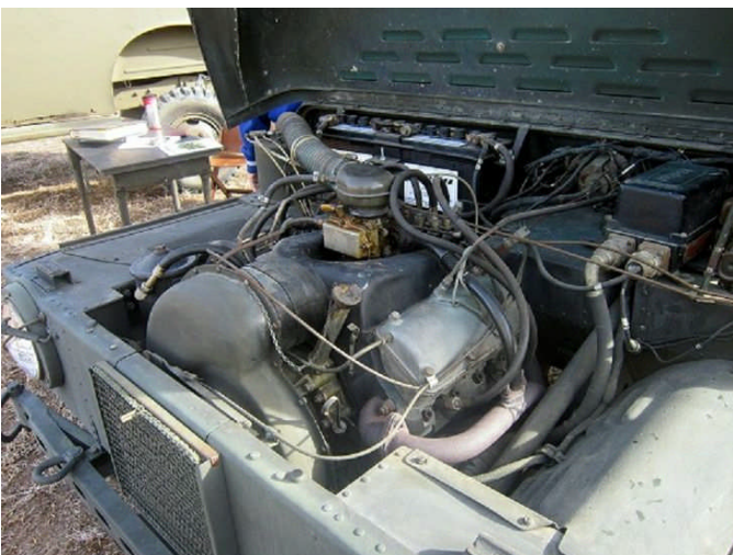
AMC Mighty-Mite V4 also used centrifugal blower.
