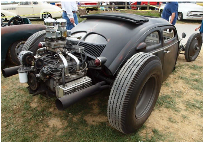
'Vair-powered Beetle with twin center-mount carbs!
