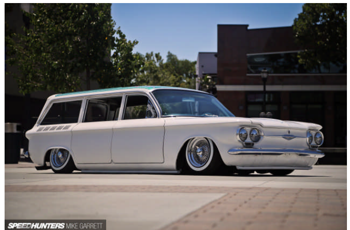
This Lakewood appears to be sitting directly on the pavement, but it has air suspension to bring it back up.
