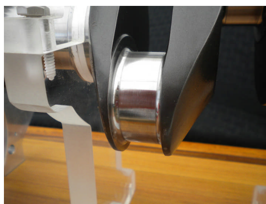
SPA Corvair USA-made billet crankshaft. The close-up on the left shows the enlarged radii at the throws.
