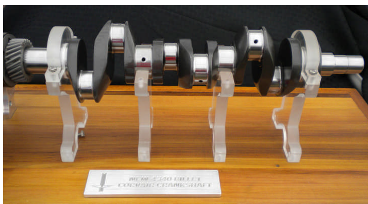
SPA Corvair USA-made billet crankshaft. The close-up on the left shows the enlarged radii at the throws.
