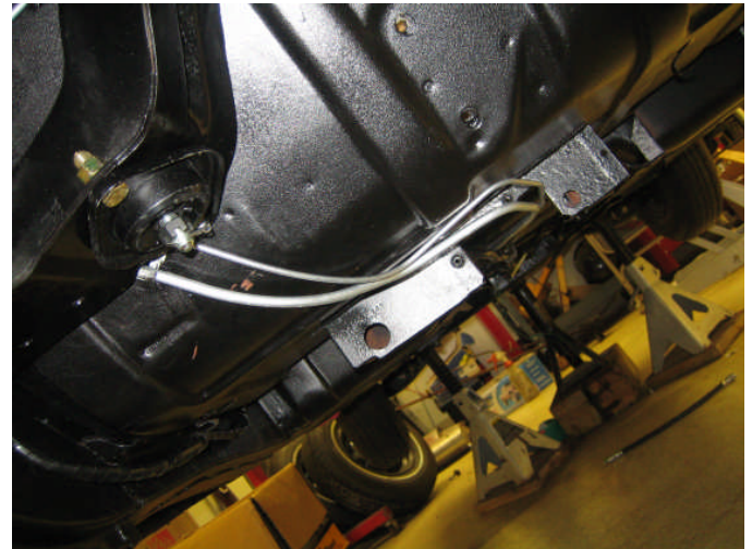
Main brake & fuel lines installed.
