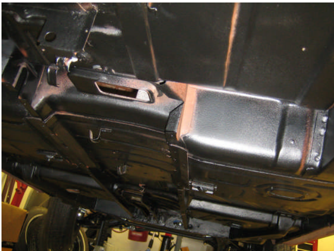
Underside awaiting second coat of paint.
