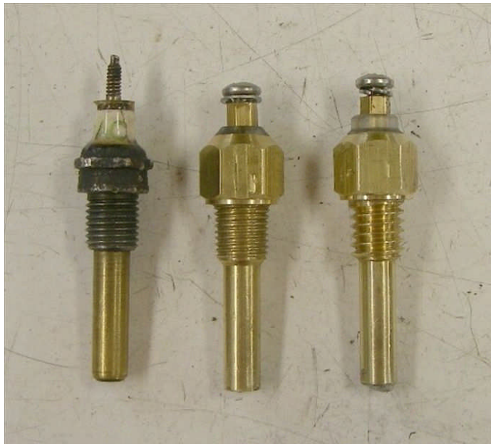
Left: Roger Parents' reproduction thermistors alongside an original A/C Delco unit. Right: Peter Faulkner's temp sensor, with electronic adapter.
