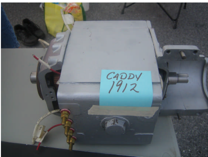
Engine starter for a 1912 Cadillac. 1st Year.
