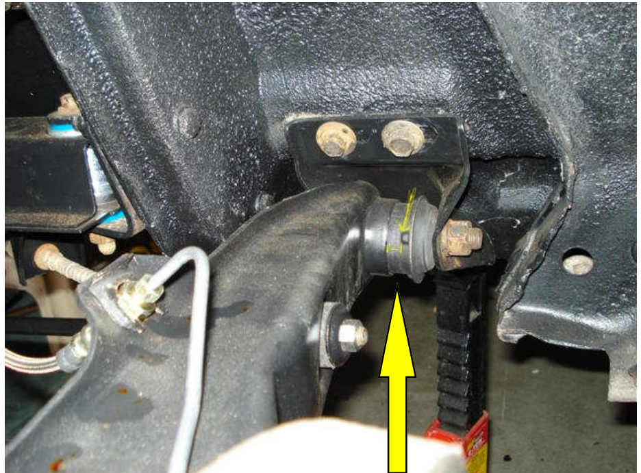
GRONK! Here is a photo showing the trailing arm of a 1965 Corvair. Notice the gap between the arm and the bushing shell.
