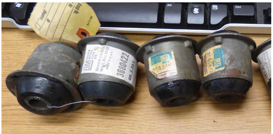
And here is a photo of the bushings. NOS GM, Part #3880422. Notice the "nubs" on the flange of the steel shells.
