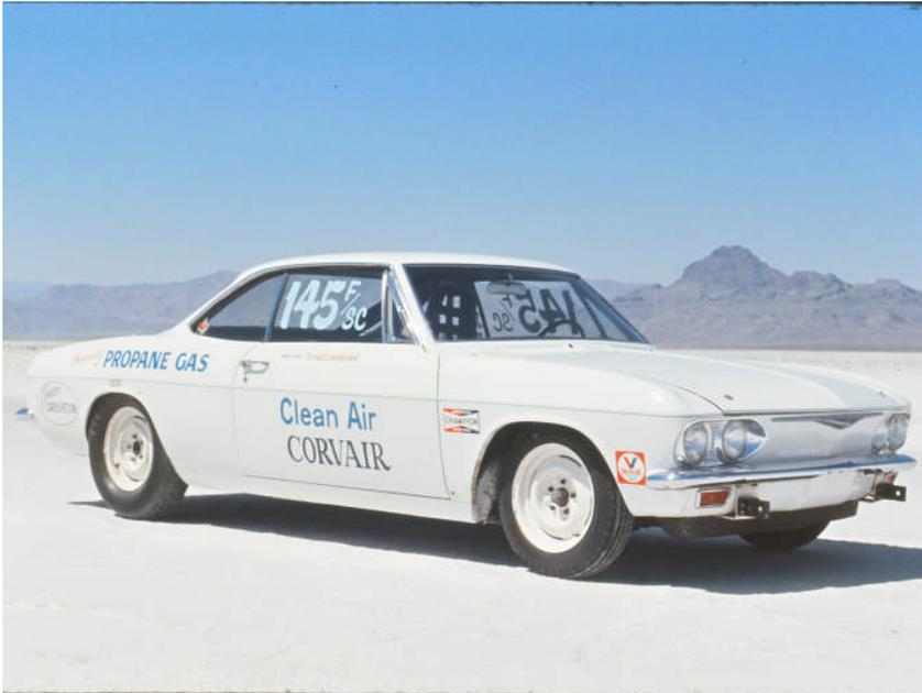
Tom Keosababian of Nevada owns this Bonneville class record holder. In 1974, the Clean Air Corvair, with its twin turbocharged, water injected, Corvair engine running on propane through a 3.08:1 final drive ratio, averaged 173.1 miles per hour in two consecutive runs.
