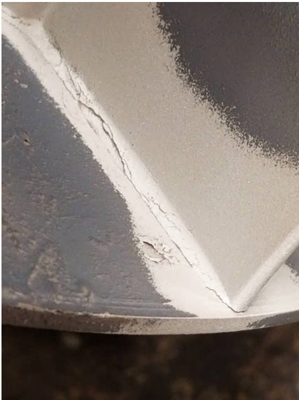
Look for cracks at the bottom edges of the blades.
