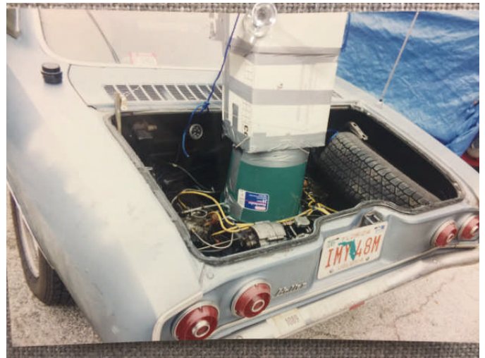
William Wynne - a big proponent of using Corvaire engines for home-built airplanes - had the engine cooling fan explode on his Corvaire while driving from Florida to New Jersey, so he McGyvered this huge air scoop to his engine to get home!
