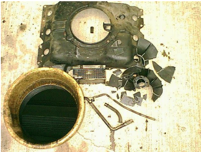
This is what they look like when they explode. Check out that collateral damage. It's messy! It even broke the oil cooler, which is why there is a big pail of dirty oil next to the turkey roaster.
