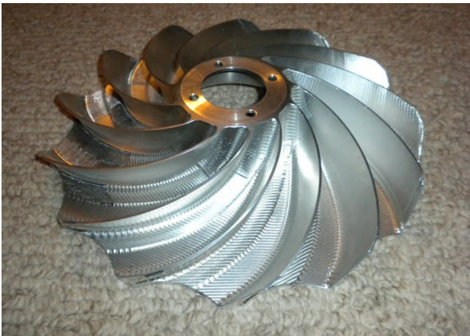
Prototype Corvair Engine Cooling Fan, by Kevin Nash.
