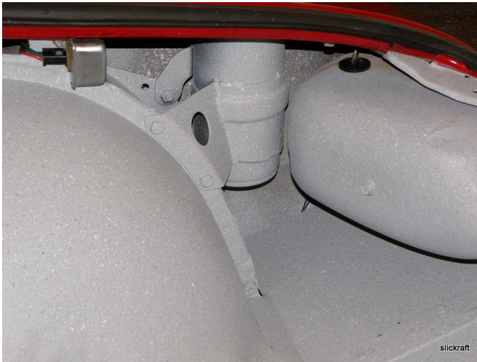
Cocktail shaker shown in the left front fender of a late-series Corvair convertible.
