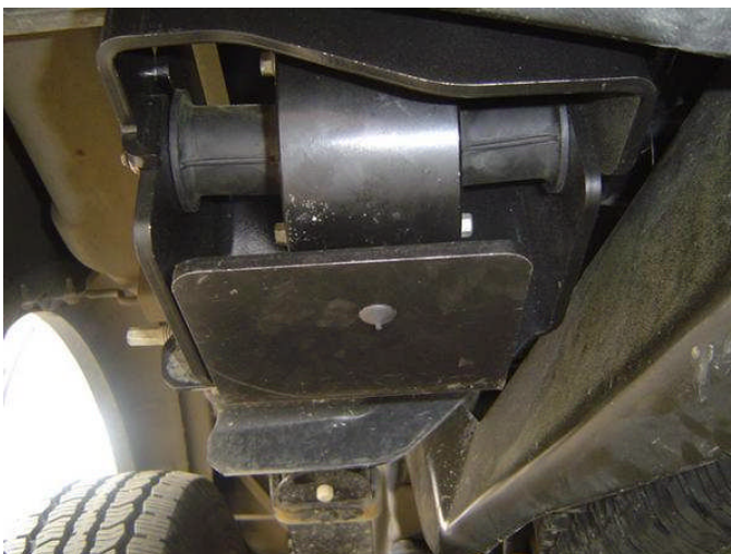
Vibration dampers are not just for old GM convertibles. Over the past ten years or so, Ford has installed them in some of their pickup trucks.
