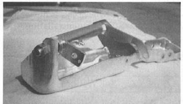
Trans support with new bracket and clutch cross shaft, ready to install in car.
