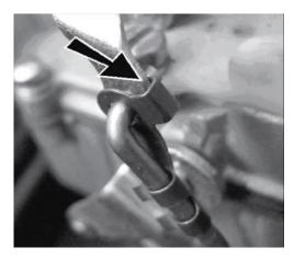
The photo above shows how the wrong clip contacts the choke lever arm preventing it from opening completely. Here the choke is mostly closed. Notice that the top part of the clip is contacting the choke arm.
