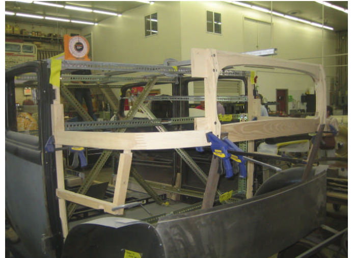
Body shop. Restoring ash wood body frame.
