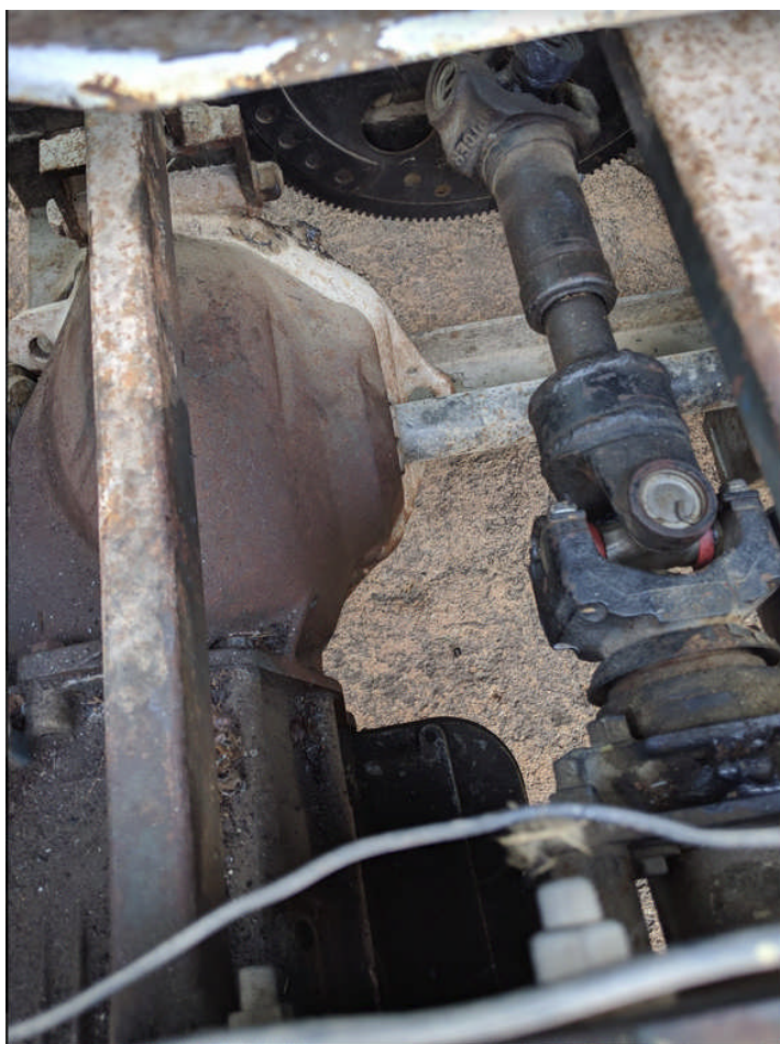
Photo below: Diff pumpkin is on the left. Drive shaft from torque converter to transmission is on the right. Axle shaft to right rear wheel is below the drive shaft.
