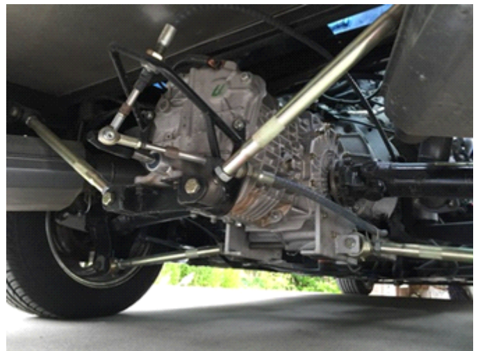
Transaxle with cable shifter setup.
