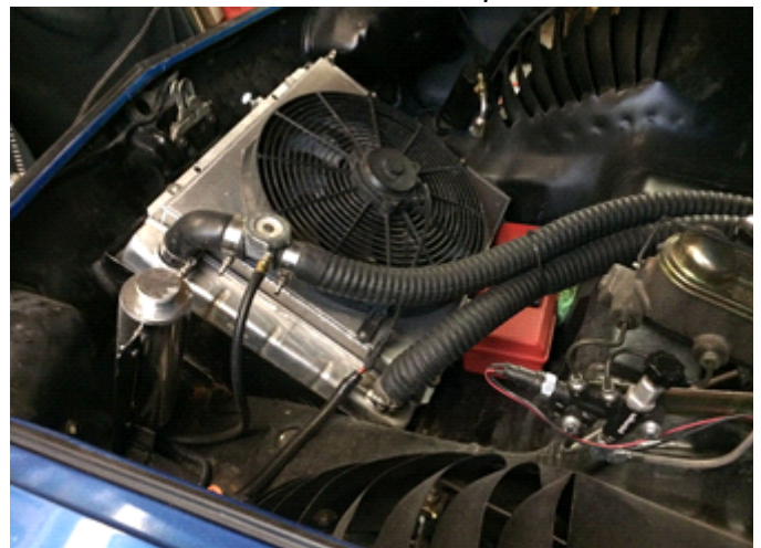
Radiator installed with electric fan.
