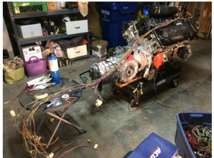
Northstar V8 mated to Porsche transaxle.
