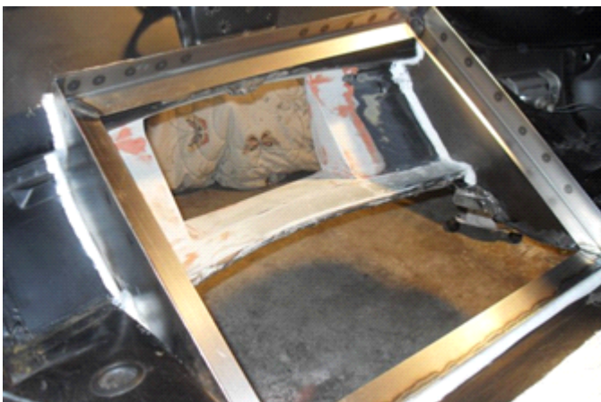
Inside the trunk: Frame for radiator.
