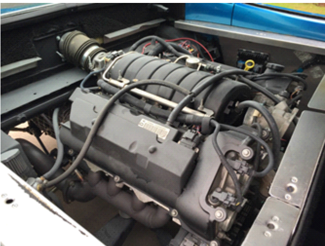
Cadillac Northstar 4.6 Liter V8 in rear seat area
