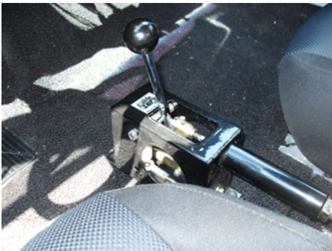
Cable shifter for Porsche transaxle.
