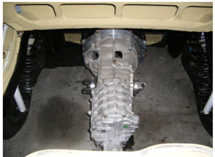
Transaxle as seen from engine compartment.
