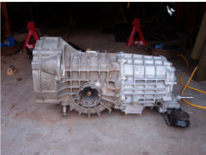
Porsche 930 transaxle with flipped ring gear, etc.
