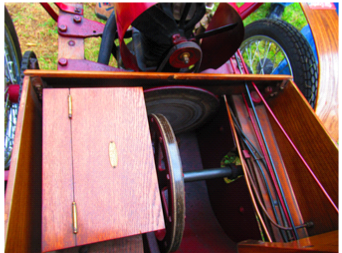
Yes, it's a CVT transmission! Two disks at 90 degrees.
