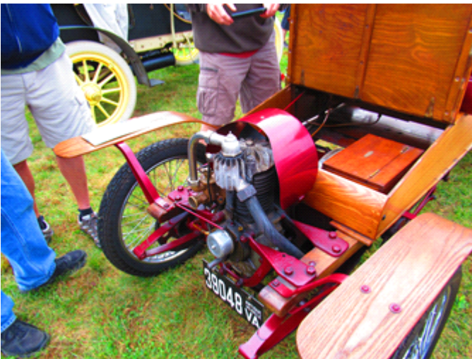
Rear-engine & air-cooled! An Orient Buckboard.
