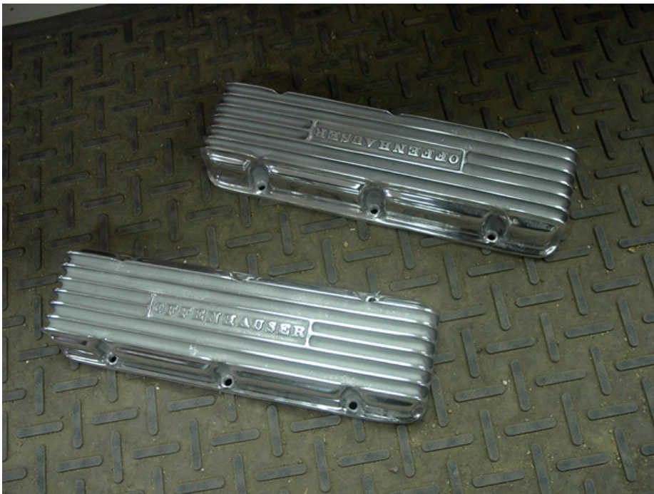
Offenhauser valve covers are inscribed with the Offenhauser name and are available in four-hole and six-hole configurations. Nice!
