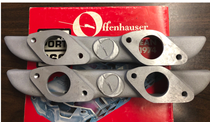
Convert your single-carb cylinder heads to twin carb, for a total of four. Carbs and linkage not included.
