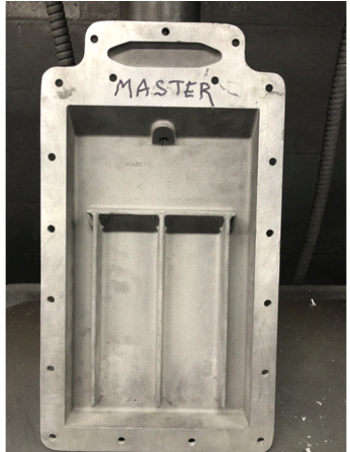
Interior of the Offenhauser oil pan. Later designs, like those offered by Otto and Clark's, have more internal fins and pins for heat dissipation.
