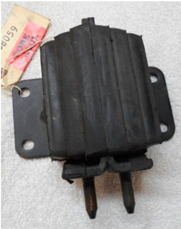
1966-69 Corvair engine mount. 2 studs. Nuts (not shown) are self-locking type, not castellated. No cotter pins.
