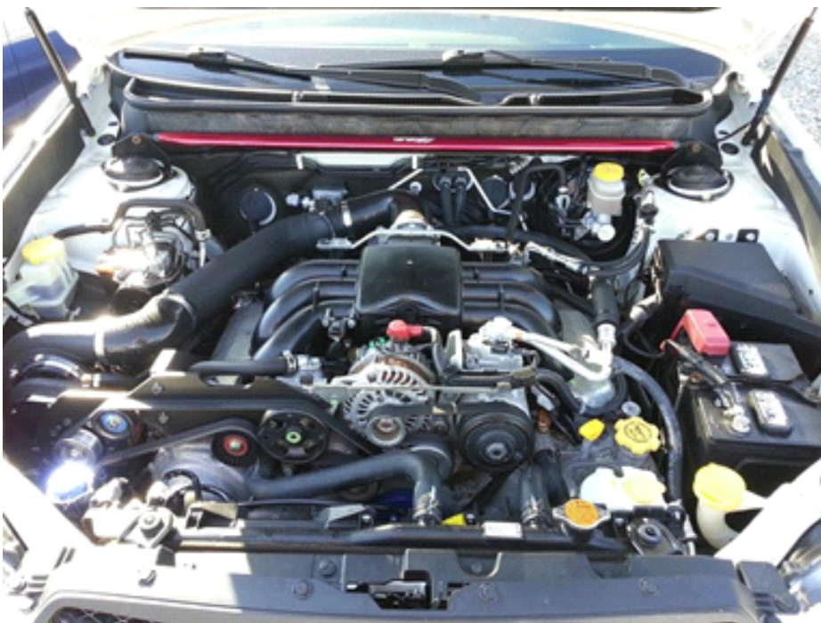
Subaru Legacy 3.6 equipped with Raptor supercharger kit.
