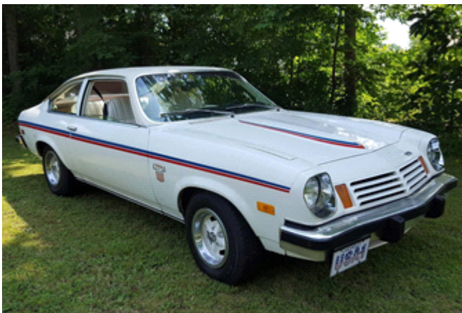
In 1974, the front styling was revised to accommodate the federally-mandated 5 MPH bumpers.
