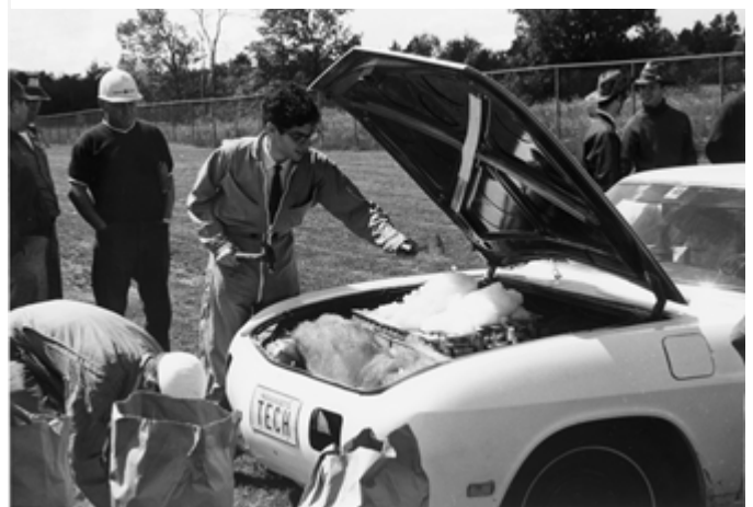
Cooling the battery packs...with ice cubes!
