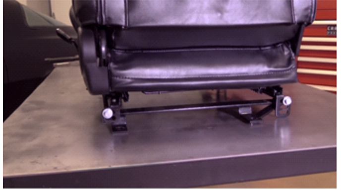
7. Adapter attached to slider brackets.
