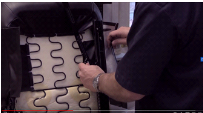
4. Bolting the sliders to bottom of seat.
