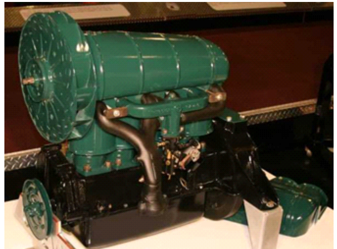
Left: Copper-cooled engine from a Delco-Light electric generator set. Right: Copper-cooled engine from the ill-fated 1923 Series M Chevrolet.
