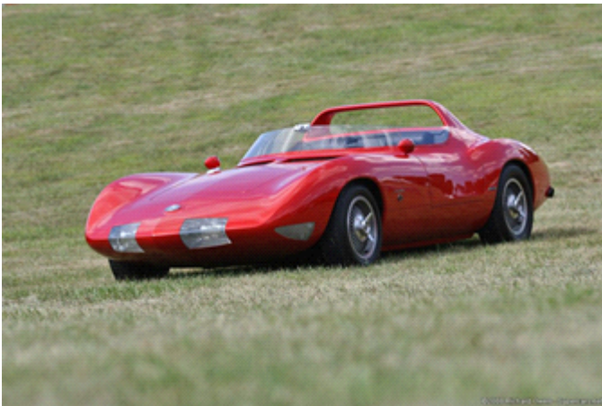
Chassis #2 underpins this Monza SS. Front fender and headlight treatment reappeared on the Chaparral 2.
