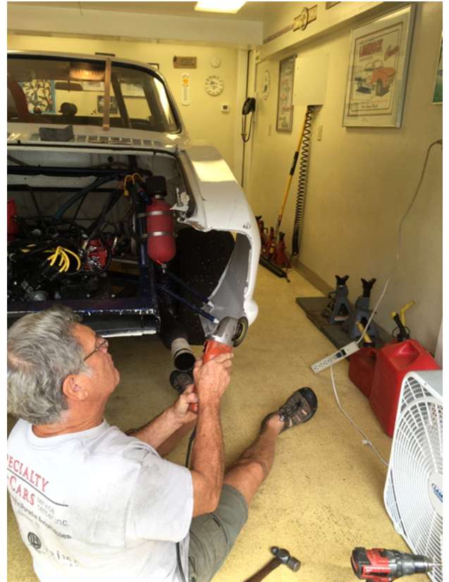
Surgery on Brian O'Neill's track car. Top-left: Sparks fly as John Egerton takes angle grinder to rear cross-member. Engine is under the blanket. Top right: John dressing the edge of fender where rear panel used to be. Bottom left: Brian and John discussing next move. Bottom right: Al Lacki with detached rear panel.
