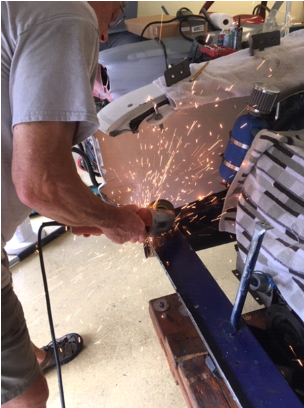
Surgery on Brian O'Neill's track car. Top-left: Sparks fly as John Egerton takes angle grinder to rear cross-member. Engine is under the blanket. Top right: John dressing the edge of fender where rear panel used to be. Bottom left: Brian and John discussing next move. Bottom right: Al Lacki with detached rear panel.
