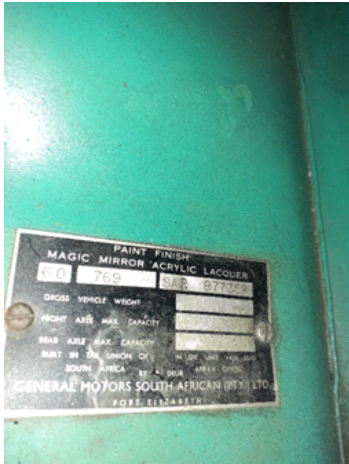
Paint finish tag has a serial number. "60 769 SAR 87735R"
