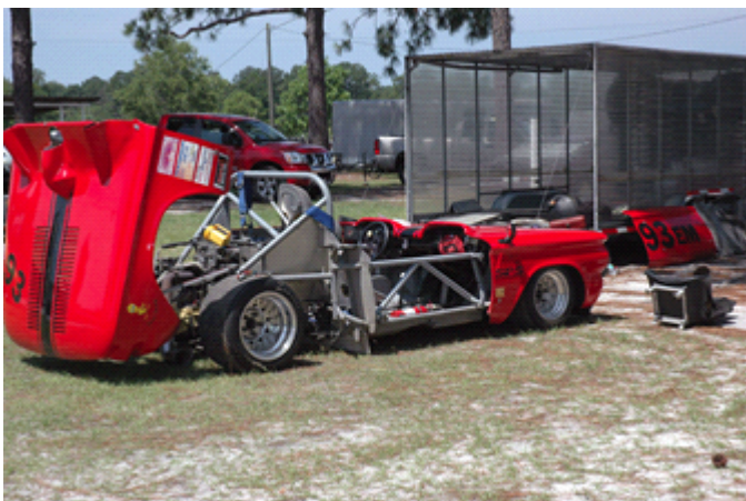
Scratch-built mid-engine tube-frame fiberglass-body
