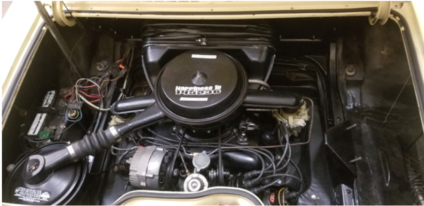
Photo #1. Desert Air Package & Oil Bath Air Cleaner options
