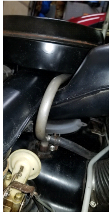
Photo #3. Special PCV Pipe installed.
