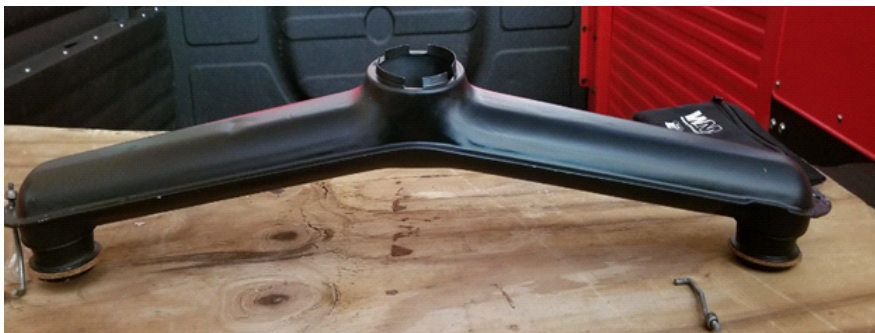
Photo #2. Crossover tube with extensions for Desert Air
