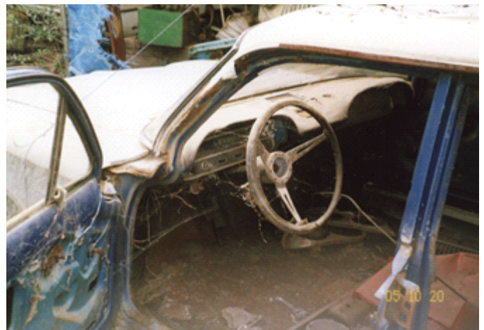
Photos 6 shows evidence that this car had been repainted sometime during its life time/ The original color, a light Horizon Blue, is evident in the exposed door panel.
