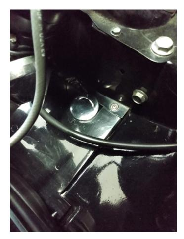
Above: Like Jeff Strausser's '66, Rich Greene's engine has that "mystery hole" in the shrouds down by the coil. Along with the fresh air hose opening in the turkey roaster, this is another opening that can lead to a hotter-running engine. He plugged it with a silver-colored plug. Look closely and you'll see it. (Rich removed the coil to take this photo).
