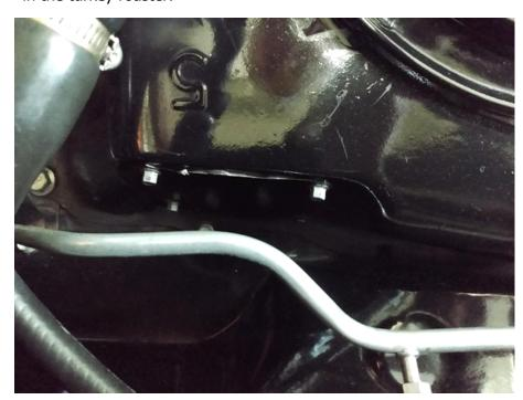
If you look closely, you can see the block-off plate he installed at the front of the turkey roaster. Secured by three tall-hat sheet metal scres, it replaces the nozzle that used to be there for the "fresh air" hose. By blocking off the opening for the hose, he ensures that no cooling air bypasses the engine cooling fins.
