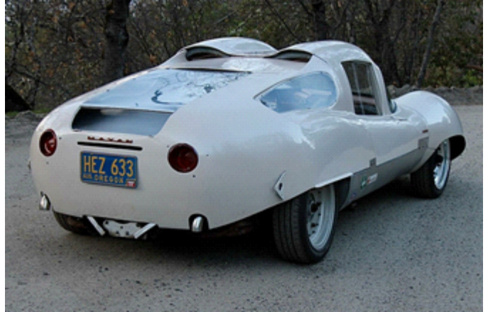
Double-bubble roof means less frontal area.
