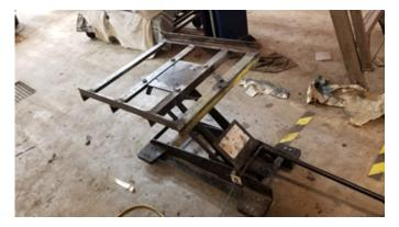
In this photo, we can see that the platform is tilted slightly. This enables Bob to remove the engine separately from the transaxle.
