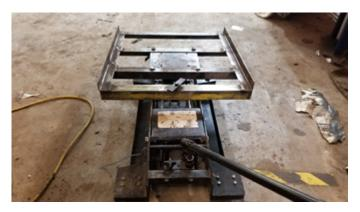
Here we have three views of Bob's engine cradle mounted on his jack. This particular jack is like a transmission jack in that the platform can tilt forward, backward and sideways.
