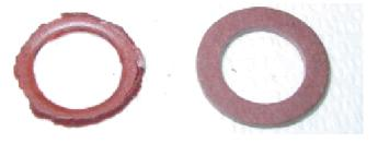
I checked my maintenance records and realized the fiber washers had not been changed on either car for almost four years. Plus the fact that the larger hard fiber gasket underneath does not seal well without the full 20 ft. pounds noted in the shop manual applied to the vertical bolt. I pulled the adapter, cleaned, checked and replaced the washer with one of my many spares. On to the Roundup.
