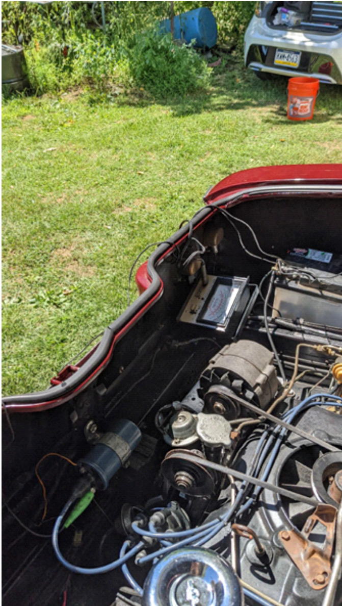
Tach & dwell meter is hooked up for final adjustment of the ignition points on Bill Geary's 4-carb engine.
