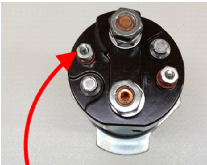
The terminal on the left is the resistor by-pass and should show battery voltage anytime the key is turned to start.
