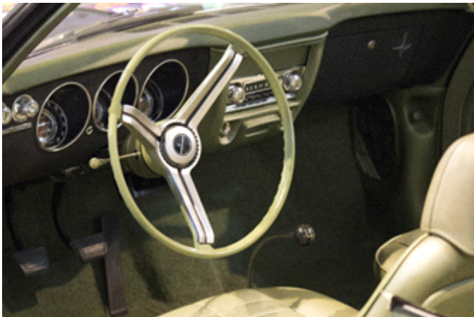
Instrument panel was largely unchanged from 1968. Note padding around the radio and ash tray.
