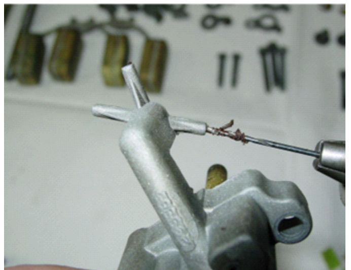
Totally plugged discharge nozzles being cleaned with a #56 drill bit.
