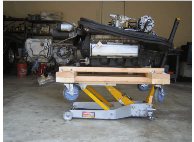
Al's homemade engine cradle, with the entire Corvair drivetrain on it
