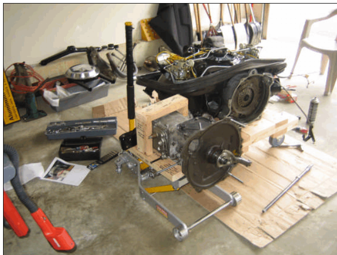
Le Heap's powertrain, out of the car and transaxle separated from engine
