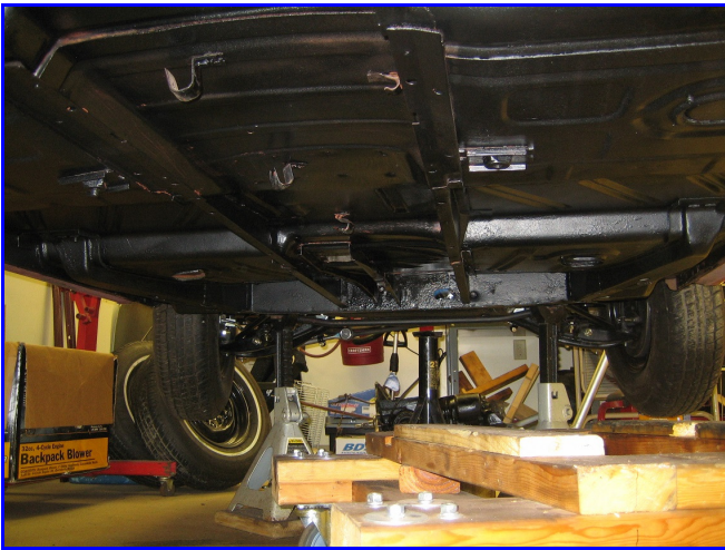
An undercarriage cleaned of 50+ years of undercoating and dirt, and repainted
