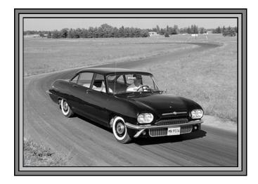
Several cars looking like this were used on public roads for cold-weather and hot-weather testing, and the substantial front grille was intended to disguise the car's engine placement from spying photographers. The cars were badged as Holdens (GM's Australian company) to further distract any media sources that might accidentally discover one of the prototypes.
